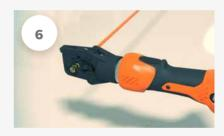
Crimp the ferrule using our pliers cod. RXA010. The deformation is achieved when the plier release.
