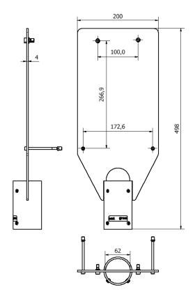
**Next Green Poleplate** 200 A is a charger mount for installation on a  $\emptyset$  60 mm pole. Poleplate is made of Swedish steel and powder coated to provide the highest durability and quality. Poleplate enables easy mounting of a charging box to a steel tube.
