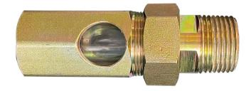
This union restriction orifice with sight glass is a conveniently usable threaded union pipe fitting and is mostly applied in a sprinkler piping test-line on alarm post or at end-of line. Orifice size has to be selected to order.
