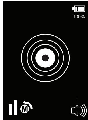
Fig. 28: Manual mode reset icon flashes in sync with reset button press
